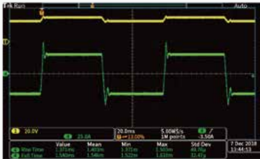
Control loop CV priority mode
